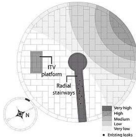
Figure 4. Micro-leaks probability on dome-roof
