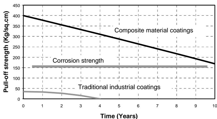
Figure 5. Pull-off strength comparison
