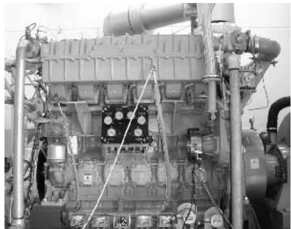
Fig.15 Side View of the New Gas Engine
