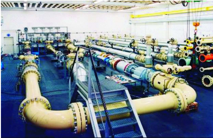
Figure 2: pignar TM : Working standards and meter test sections
