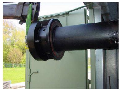
Picture 4 shows the annular gap of the vortex tube.
