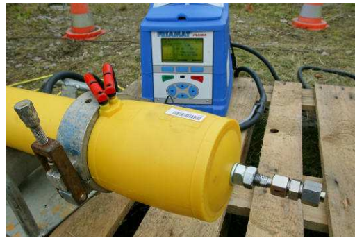
Fig.7: electro-fused end cap with gas connection
