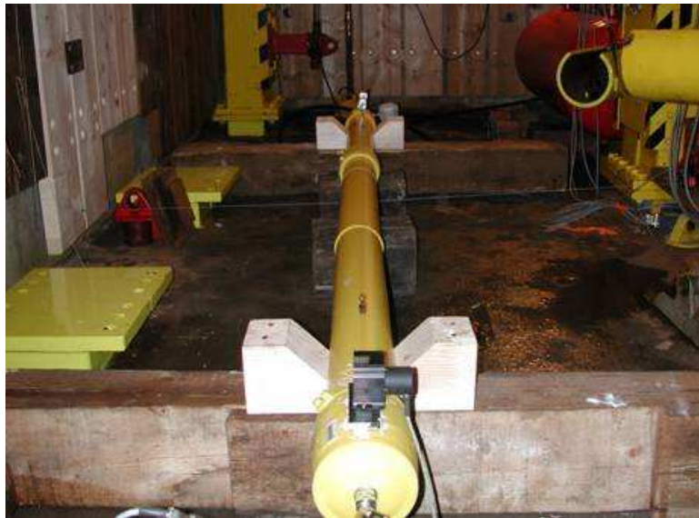
Fig. 4: VESTAMID gas pipe D110, SDR-11, with joints, quick burst test,
