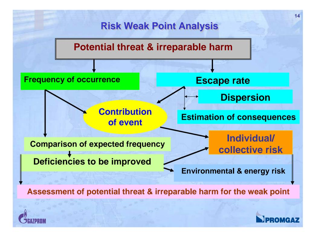
Concept of Assessing Risk in Heat, Power, Hot Water and Steam Production by SUS CCU: Calculation Methodology
