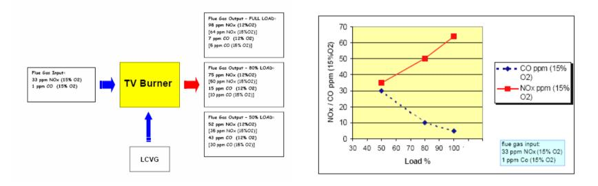
•CO and NOx emission dependent on load•Optimum design for burnout of fuel but NOx increases with load
