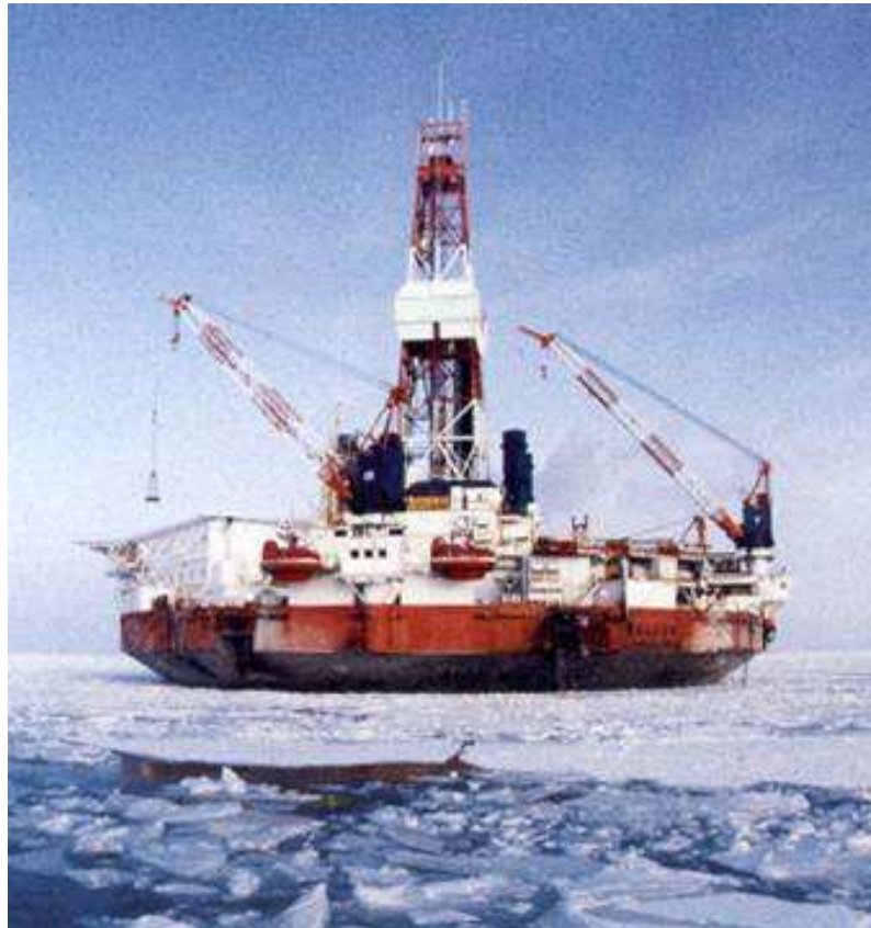
Kulluk ice resistant drilling rig in Beaufort Sea
