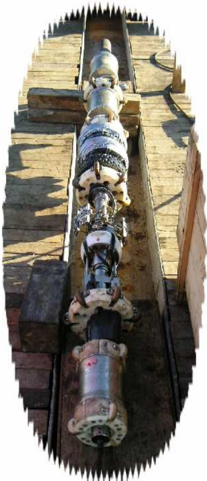
← ICP – inspection tool
