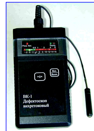
EDDY CURRENT CRACK DETECTOR VK-1 FOR MONITORING OF THE CRACK LOCAL DEPTHS
