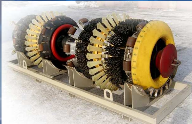
TWO SECTION MAGNETIC PIGS WITH BY-PASS UNITS LONGITUDINAL MAGNETIZATION
