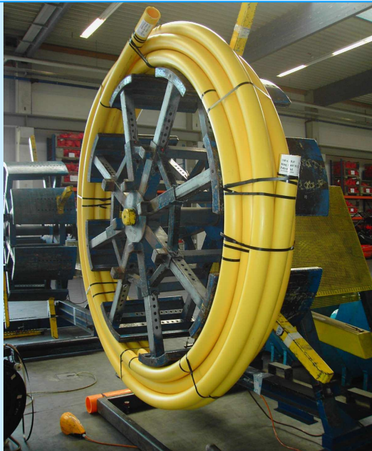
Coiling of D100 SDR-11 pipe on 2.7 m drum!
