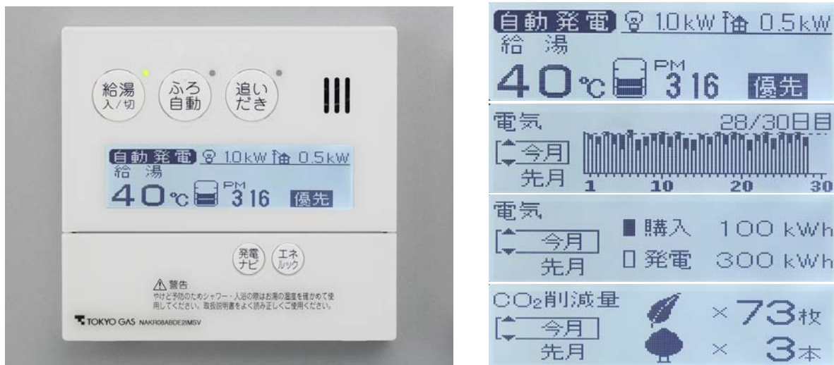
Figure 2: The control device displaying a history chart of past electricity generation
