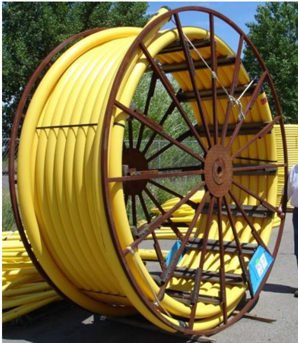
Figure 4 – 4" PA12 pipe supplied in both coiled and 50' long sticks
