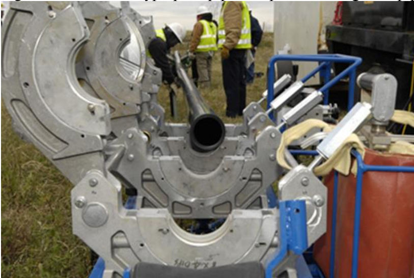
Figure 2 – Standard butt fusion equipment used to connect PA11 pipes together
