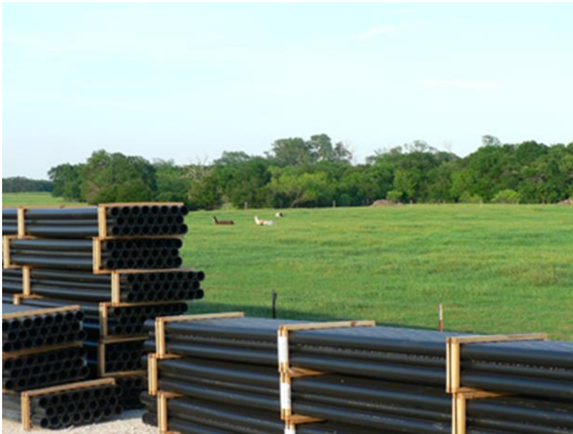
Figure 1 – 4” PA11 Hyperplast pipe to replace existing steel piping system
