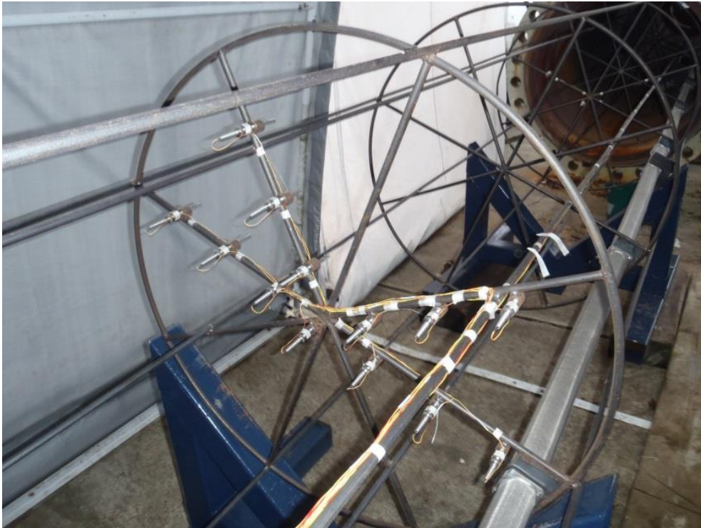
Figure 4: Photograph of the metal frame showing the thermocouples and distributor.
