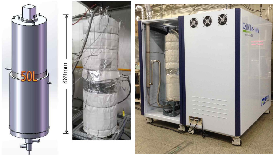
Figure 4 the 10kW-class reformer developed by KOGAS and its application to fuel cell system
