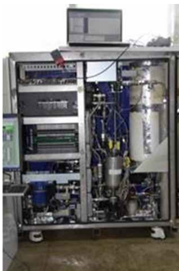
Figure 2. The performance of 1kW-class reformer developed by KOGAS
