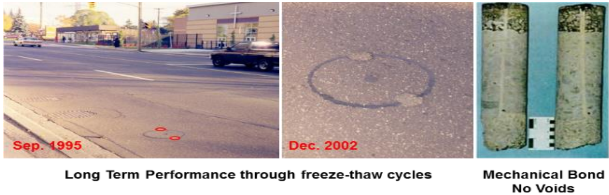
Figure 7. Test cores cut through the kerf on each side of a reinstated core show complete penetration of the bonding compound (thin grey line in the center) through the asphalt and concrete layers of the core. Long term performance via mechanical waterproof joint created by bonding compound.
