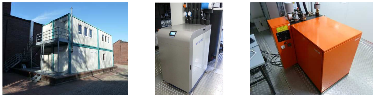
Figure 1: Test facility, adsorption chiller and the CHP engine
