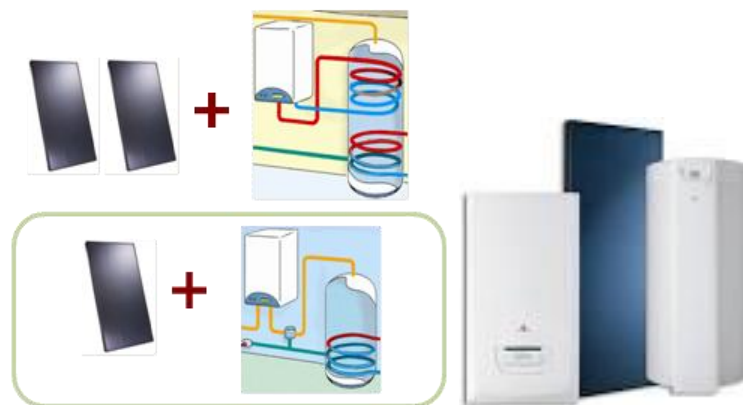
Figure 5: The optimized solar thermal heater, compared to a classical one.
