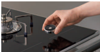
The twist switch can be detached. In an emergency, gas can be shut off by detaching the twist switches.
