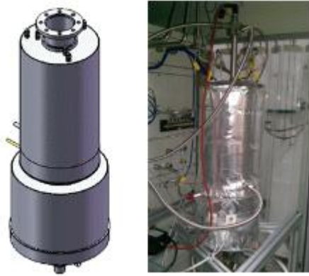
Fig. 4 Reformer Design and Manufactured reformer
