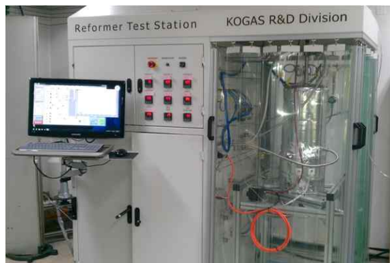
Fig. 5 Test station of 5Nm 3 /hr Reformer
