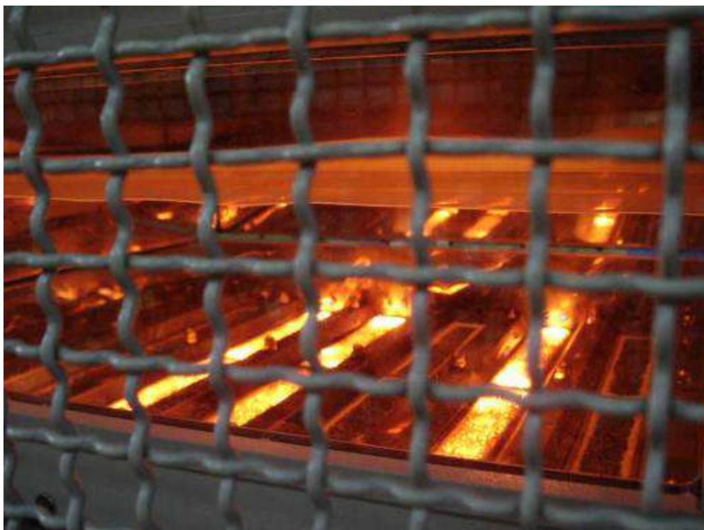
Figure 7 – Plastic film being heated by gas radiant burners
