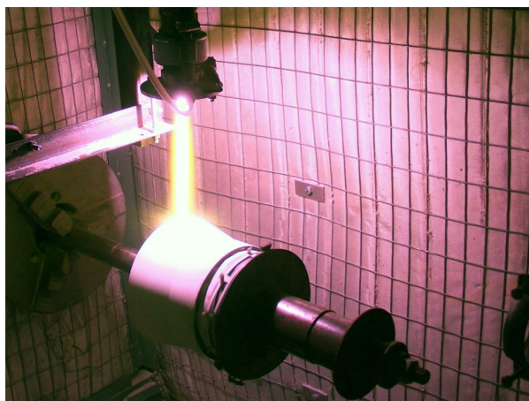
Fig. 8. The process of plasma spraying of thermal barrier coating on the part of the pyrolysis reactor.
