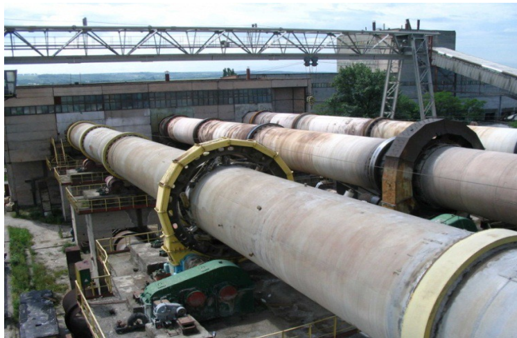
Fig.5. Rotary kiln fueled by sunflower husk.
