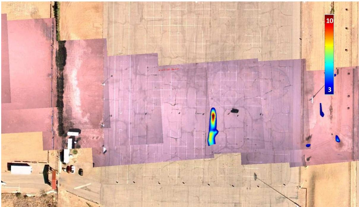
**Figure 11: 1100 scfhr plume image with integrated column thicknesses (in mm)**
