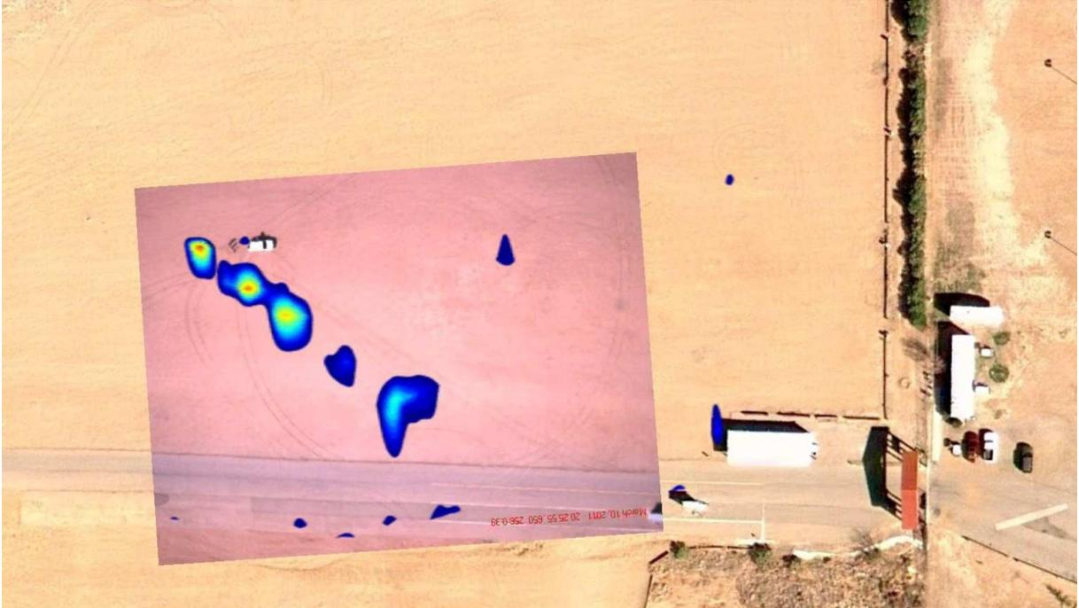
**Figure 10: 1100 scfhr plume image under gusty wind conditions**
