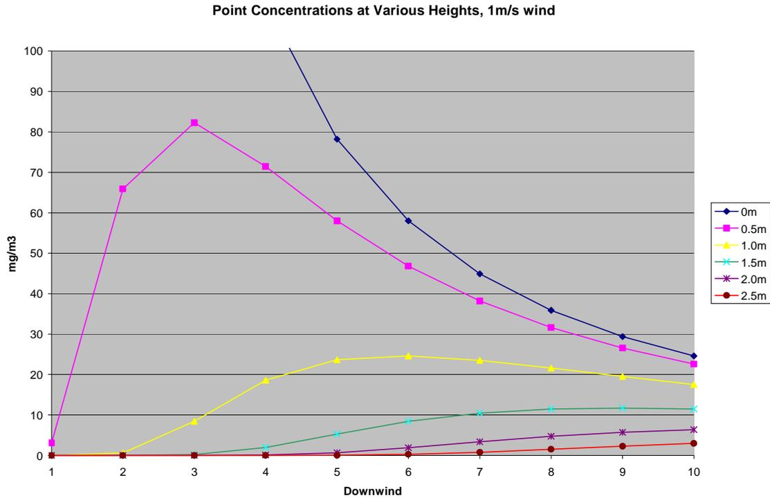
**Figure 6: Centerline downwind concentrations at various heights**
