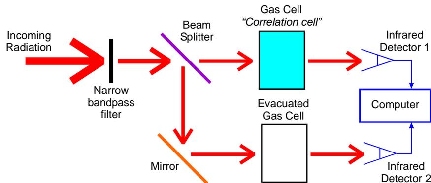
Figure 2: GFCR Conceptual Diagram
