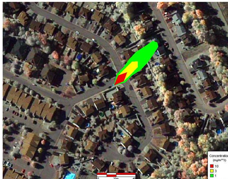
**Figure 5: Plume simulation contours**
