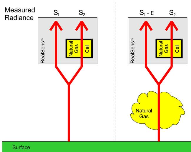
**Figure 3: GFCR Measurement Principle**
