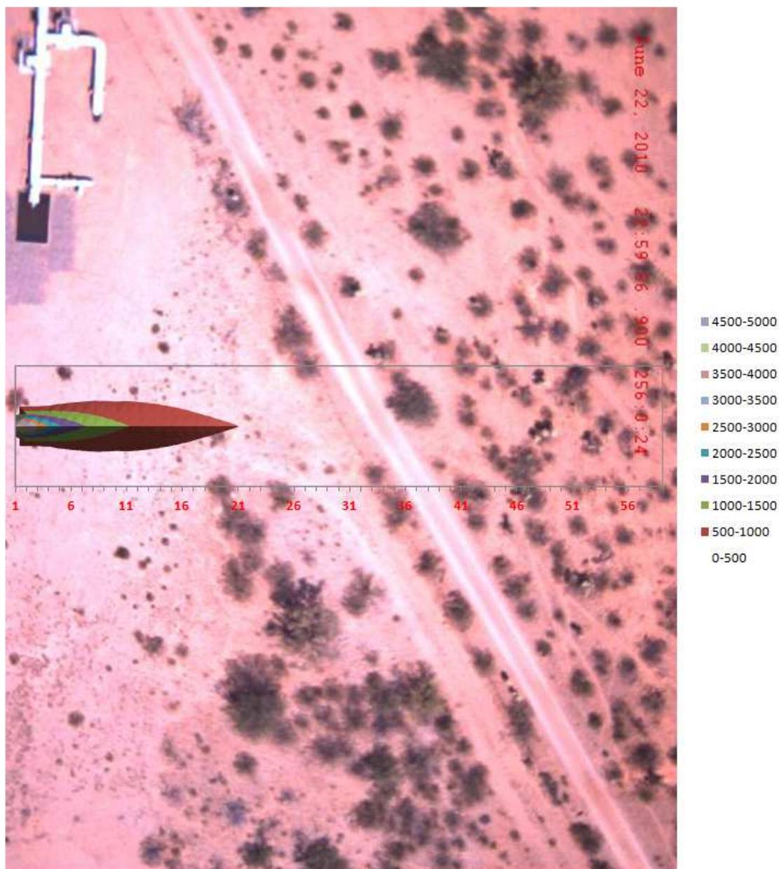
**Figure 8: 2D plume image with integrated column thicknesses (in  $\mu\text{m}$ )**
