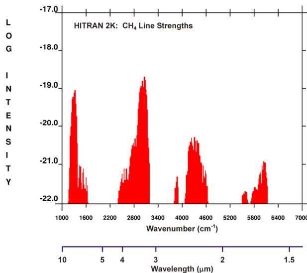
Figure 1: Methane Spectral Absorption Bands
