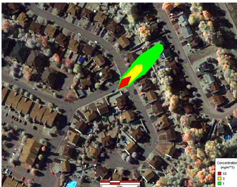
**Figure 5: Plume simulation contours**
