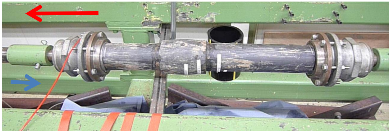
Figure 9 – Test setup for testing the full-end-load resistance of the joint. The red arrow indicates the pull direction and the blue arrow the inlet for the air needed to keep the system at a constant gas pressure of 30 mbar.
