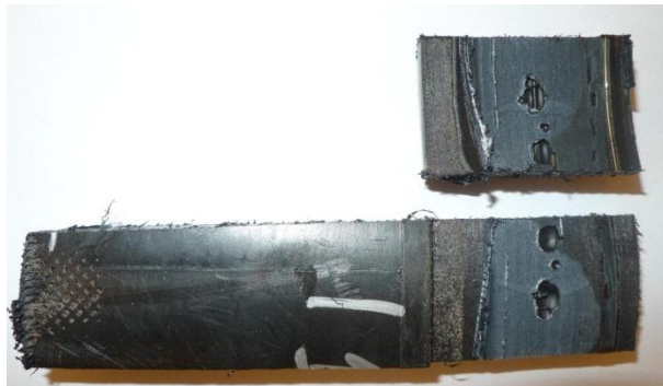
Figure 5 – An example test sample after the Peel decohesion test on the Rollmaplast couplers. Cavities were found at the welding zones in many of the samples.
