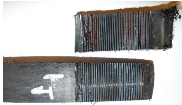
Figure 6 – An example test sample after the Peel decohesion test on the Mannesmann couplers. There is almost no connection possible between the coupler and PE pipe due to the high density of wires at the welding zone.
