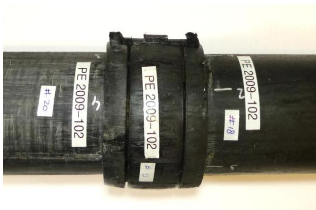
Figure 1 – Rollmaplast coupler with distinctive groove on the outside
