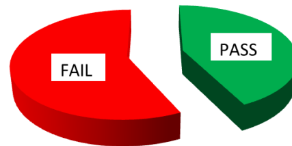
Figure 8 – Results of the Peel decohesion test on Mannesman couplers. Of the 14 investigated first generation PE electro-fused Mannesmann joints, only 6 passed the peel decohesion test.
