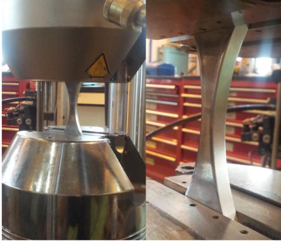
Fig. 7 Fatigue tests of curved plate specimens
