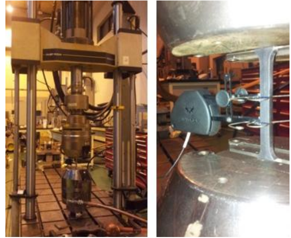
Fig. 5 The hydraulic test machine and extensometer
