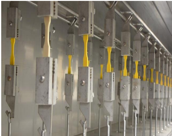
Figure 6 – Constant load experiments on PVC samples
