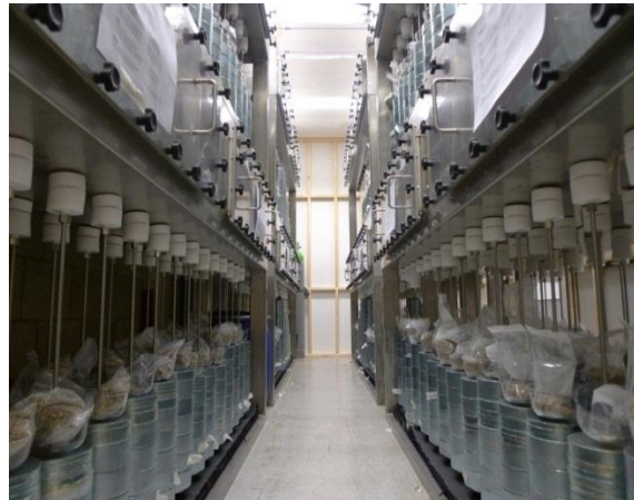
Figure 7 – Full-scale setup used to determine the effects of sustainable gases on polymeric materials
