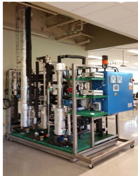
Figure 4. Bench-scale Closed Loop Reactor at Akermin's Research and Development Facility
