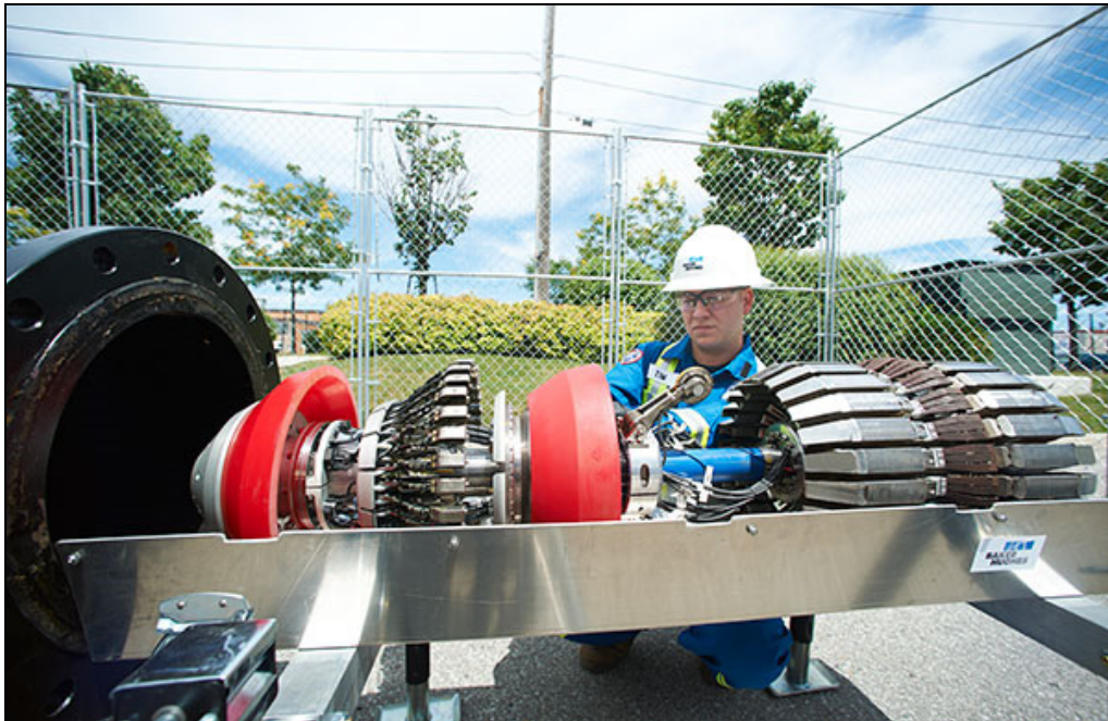
Figure 1: a 16" Inspection pig, photo courtesy of Baker Hughes PMG
