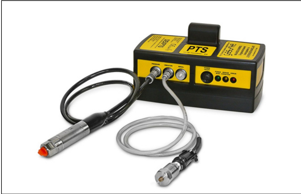
Figure 6: Field unit with pressure and vibration sensor
