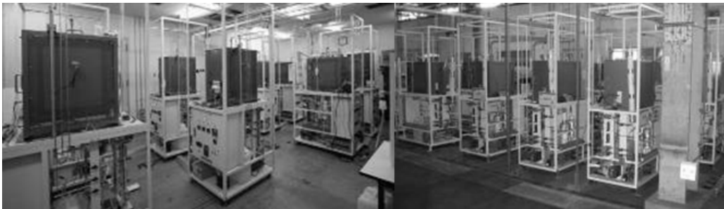
Figure 3 Stack durability test units.
