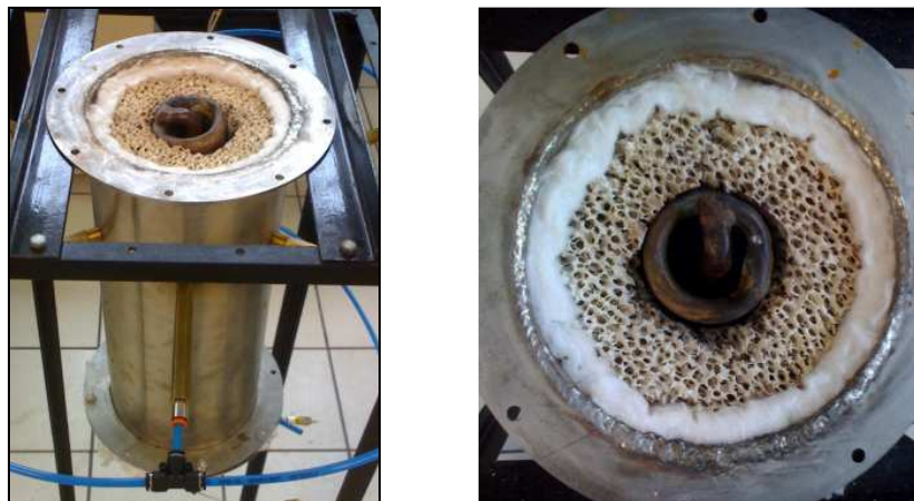
Figure 3 - Photo of the burner open surface and the coil positioned in the center of the porous medium.
