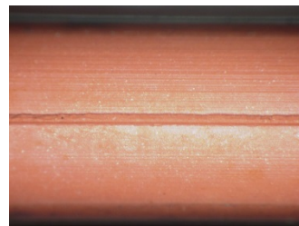
Figure 2(c). No cracks, voids, or substances were observed on the surface of FKM1 aged in water with 5 ppm chlorine for 18,000 h.
