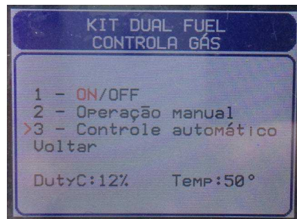
Figure 17 - Control of natural gas interface
