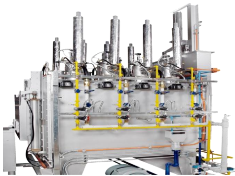
Figure 4: Single-ended RT Burner Installations in Furnace Body
