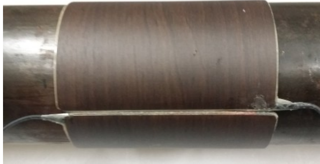
Figure 4. Installation of magnetostriction type sensor
