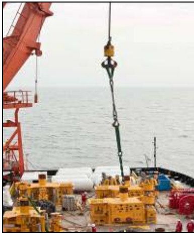
Figure 4. Lifting of the subsea tree
