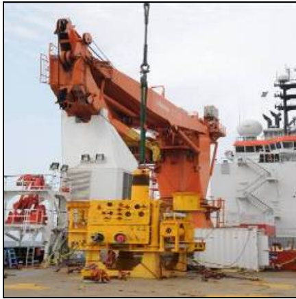
Figure 3. Preparation of the subsea tree in the vessel deck
