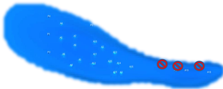
Figure 2. Schematic for injection and production wells in the 2nd scenario.
