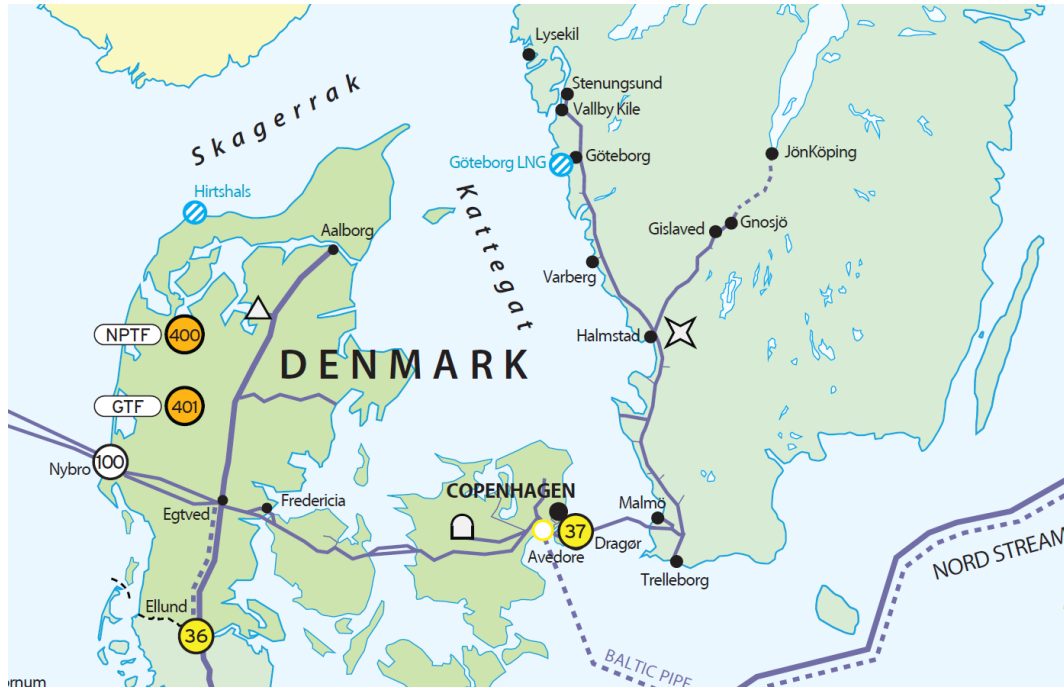
Figure 1. ENTSO-G map of the gas transmission network of Denmark and Sweden (Source: ENTSOG 2014).
