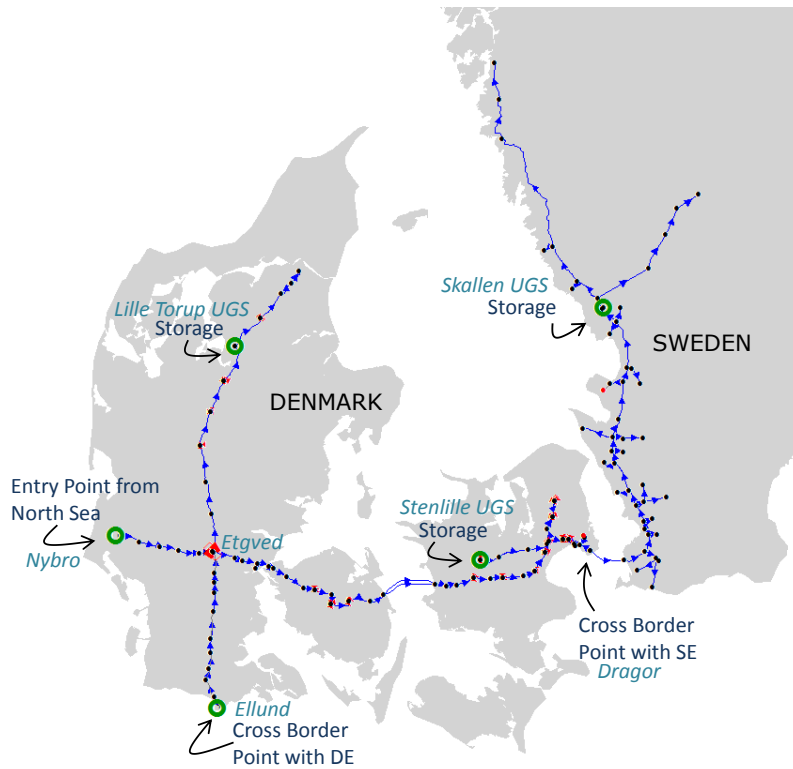
Figure 2. Gas network model of Denmark and Sweden built in SynerGee® Gas software.
