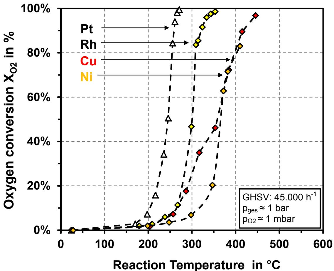
**Fig. 6: Comparison of different catalysts for the conversion of oxygen by oxidation of methane**
