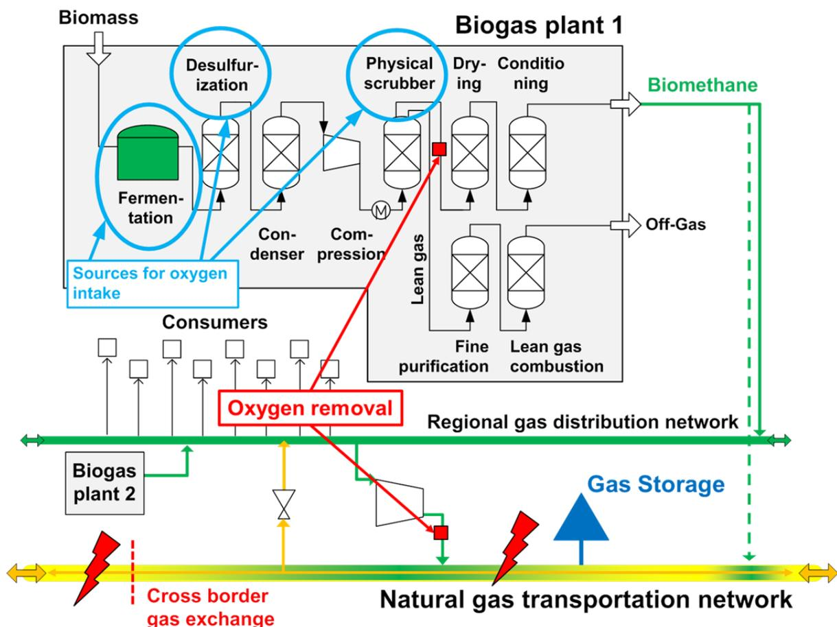
Fig. 1: Overview over a typical biogas plant setup, points of oxygen intake and spreading of the oxygen load in the gas grid infrastructure (■: possible installation points for O<sub>2</sub>-removal units)
