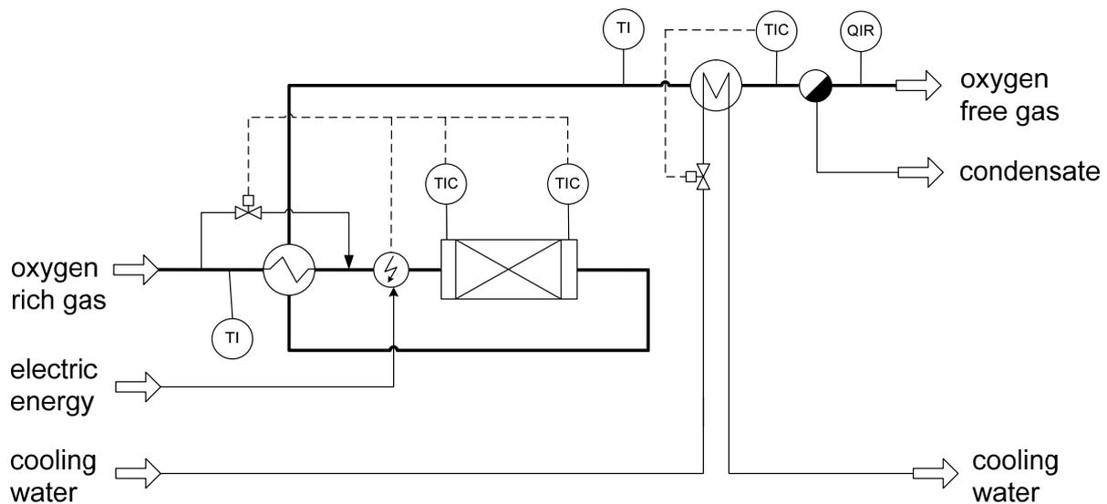
**Fig. 7: General setup for oxygen removal by catalytic oxidation processes**
