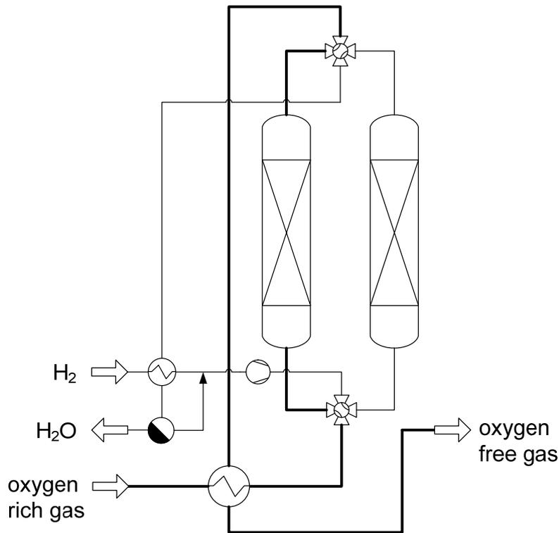
**Fig. 2: Flow scheme of an adsorption based process for oxygen removal**
