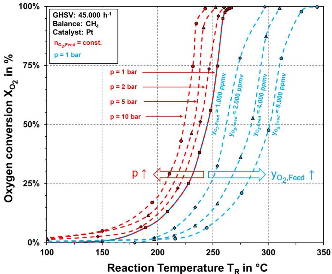
Fig. 4: Oxygen conversion in the lab scale test rig at Engler-Bunte-Institute as a function of feed composition and system pressure
