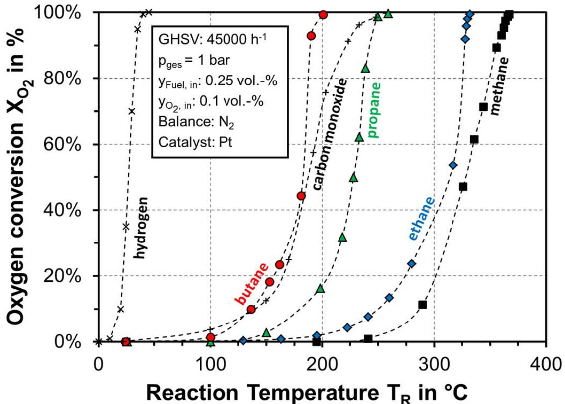
Fig. 5: Comparison of the activity of different fuel gases for the conversion of oxygen
