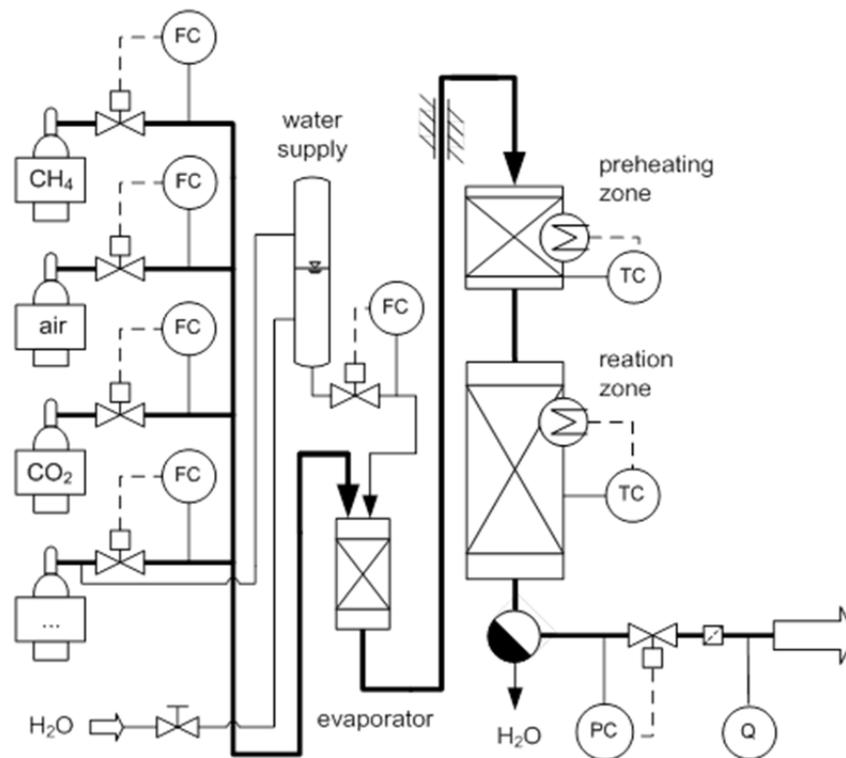
Fig. 3: Flow scheme of the experimental setup used in this work
