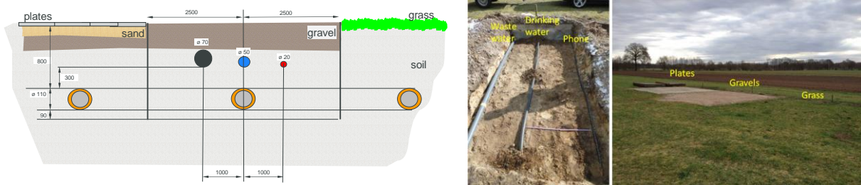
Figure 7. View and picture of the urban test rig of E.ON: gas injection was performed in the middle compartment to assess the influence of the buried pipelines
