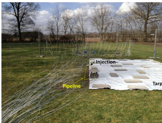
Figure 5. Picture of the TF2 rural test rig in the configuration for gas migration in soil study
