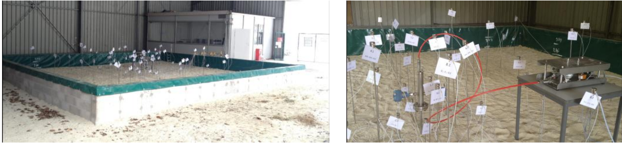
Figure 2. Pictures of the GDF SUEZ homogeneous test rig with the device set up for the characterization of the gas migration in soil.
