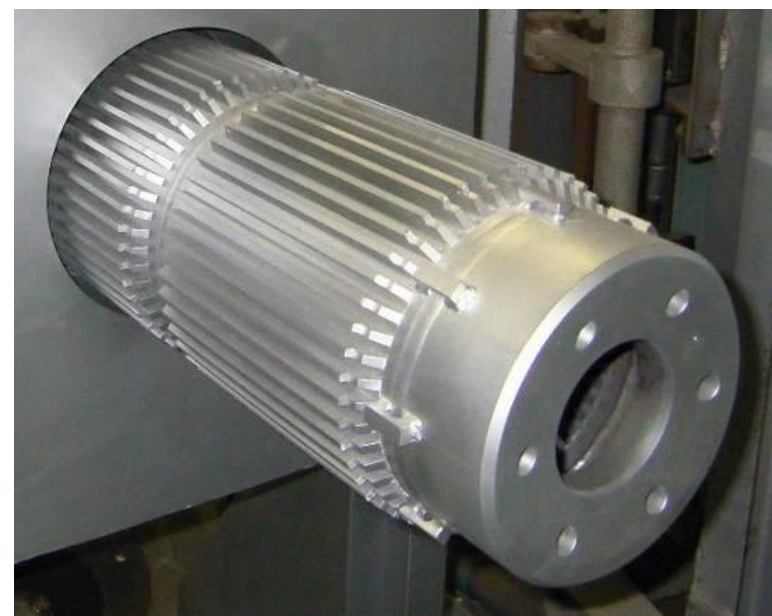
Top of Heat Exchanger
