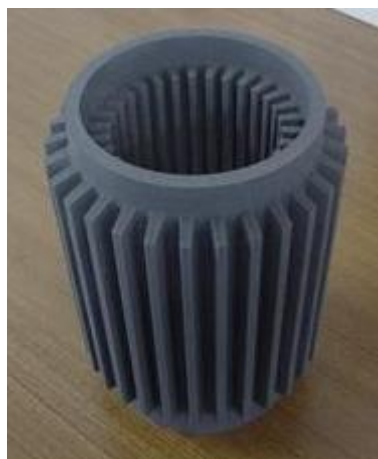
Lost wax model by 3D printing ( resin )
