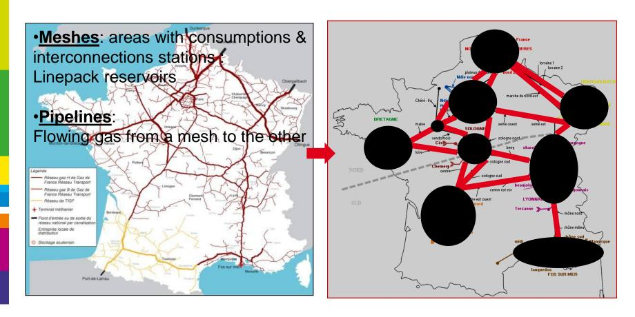
A trajectory = hourly flows at each end of pipes + storages + LNG
