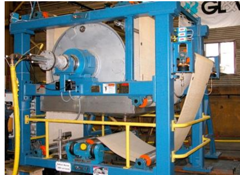
GTI Drum dryer demonstration in paper drying facility
