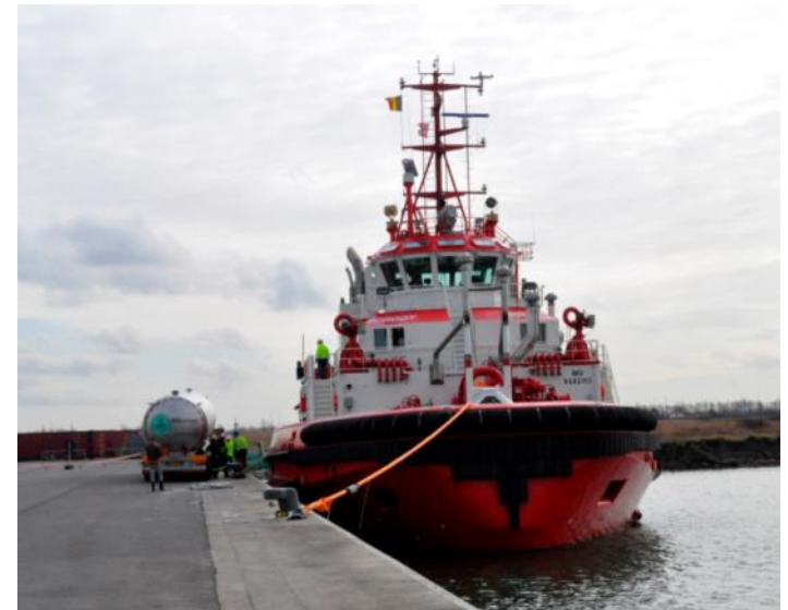
Bunkering of 1st LNG-fuelled tugboat M/T Borgøy in the port of Zeebrugge
