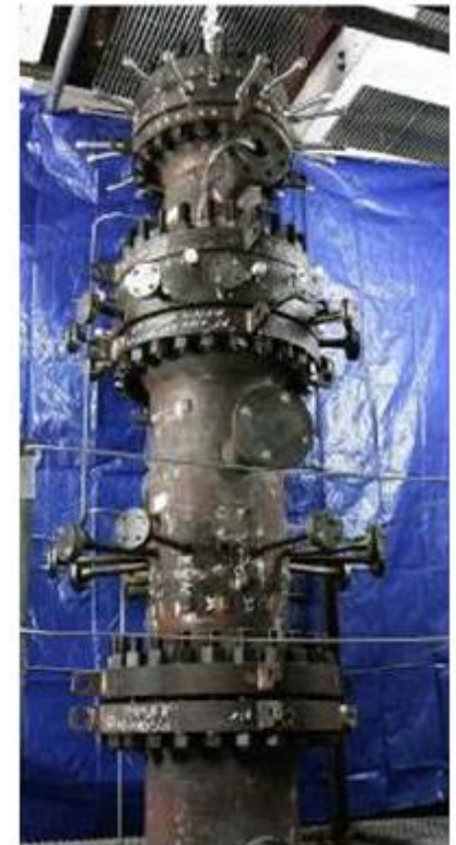
POx Development Combustor at GTI
