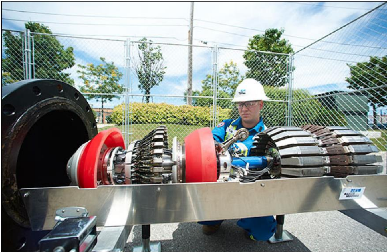
16" Inspection pig, photo courtesy of Baker Hughes PMG
