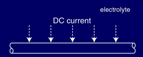
CP reduces or eliminates the corrosion of a pipe surface by making that surface the cathode of an electrochemical cell, with a DC current flowing through electrolyte to the pipe surface.
