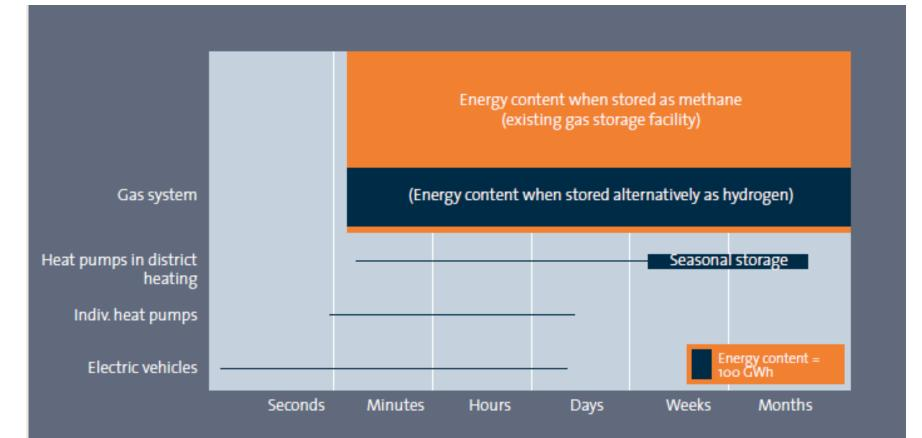
Figure 1-8: Energy content (electricity input) of different storage types in the energy system. The orange areas show the size of the potential energy storage. For gas, the small black box indicates the content if the gas is stored as hydrogen rather than methane.
