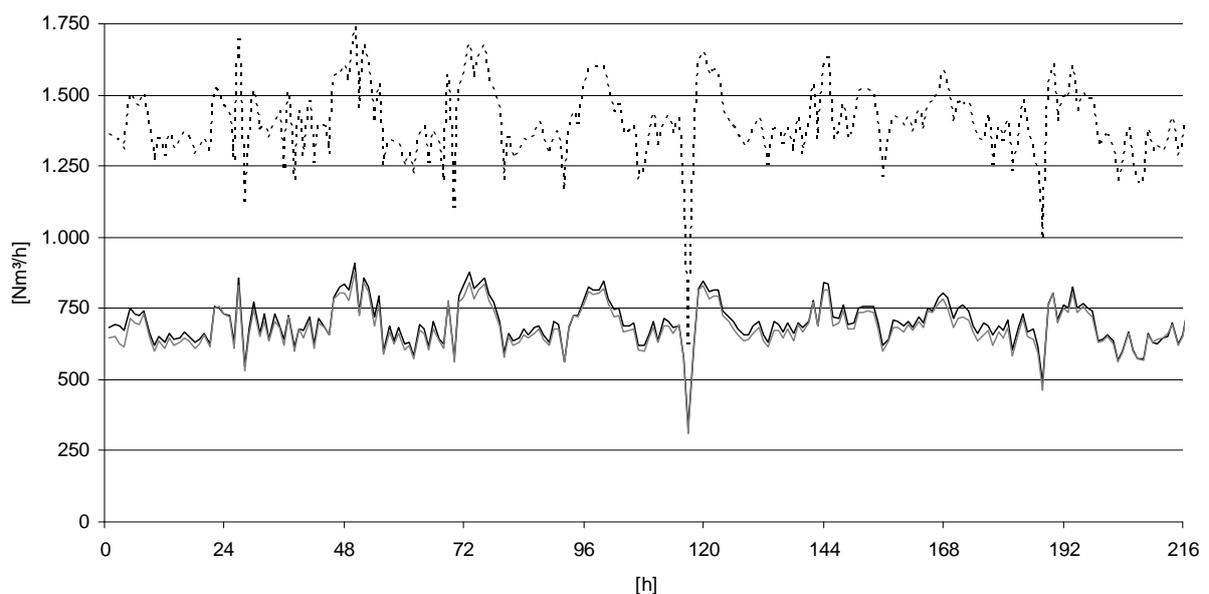
Figure 10: Normalised volumetric flow of raw biogas after secondary digester 1 (black line), after secondary digester 2 (grey line) and in the collection pipe (dotted line).
