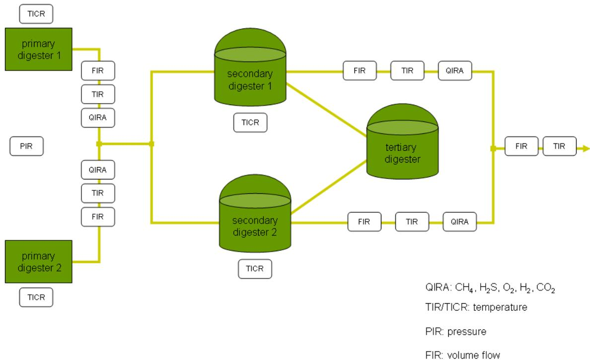
Figure 3: Biogas flow pathways and selected meters of the production line 1 of the Schwandorf biomethane plant
