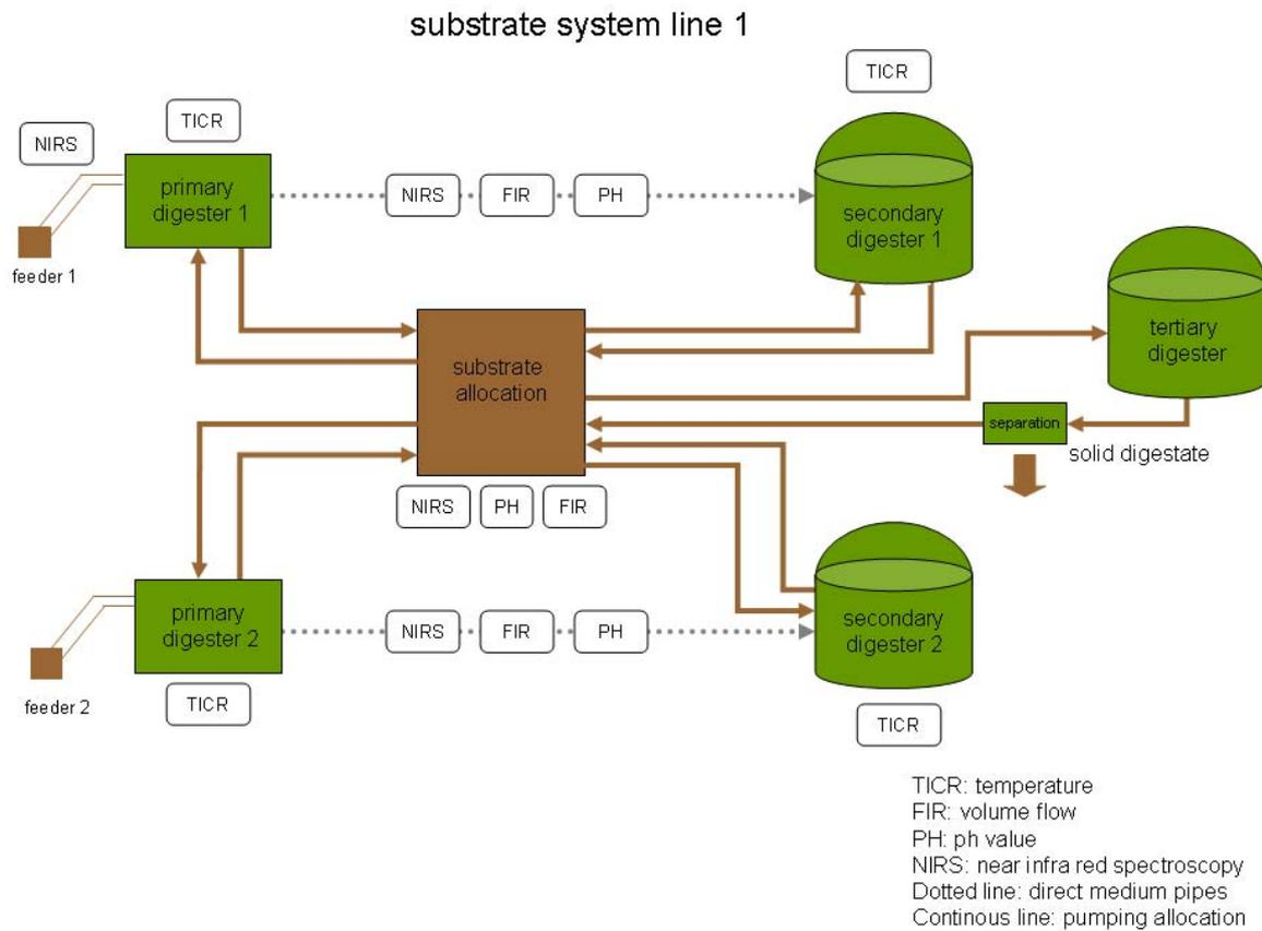
Figure 2: Substrate flow pathways and selected meters of the production line 1 of the Schwandorf biomethane plant.
