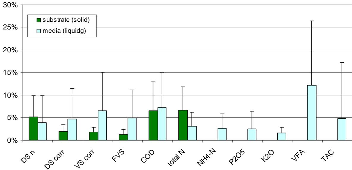
Figure 9: Mean deviation of NIRS results compared to their chemical references ( $n_{\text{substrate}} = 10$ ,  $n_{\text{media}} = 29$ ).
