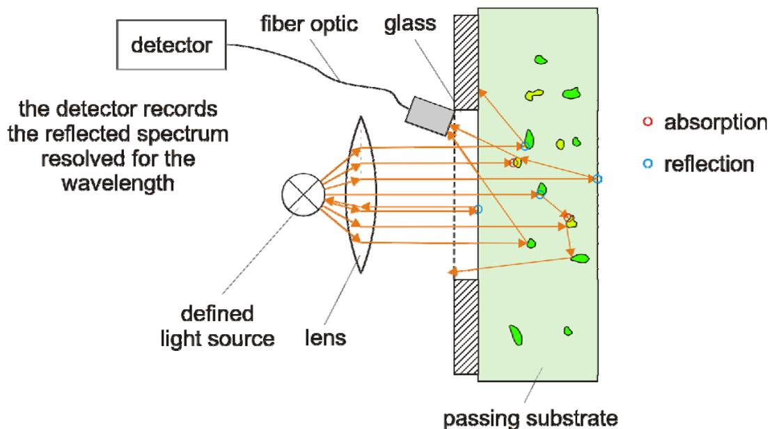
Figure 4: Measuring principle of NIRS (drawn after [6])
