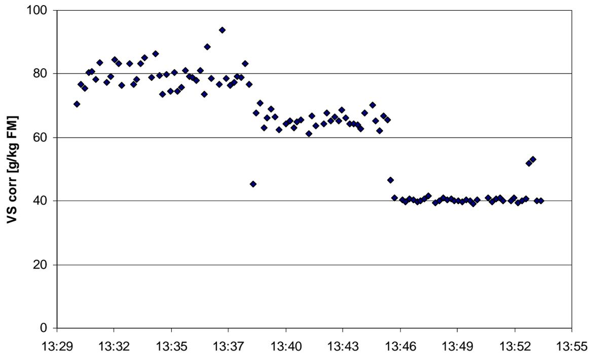
Figure 8: Volatile substances ( $VS_{corr}$ ) in the central substrate allocator unit. The media were switched every 4-7 minutes starting with primary digester 1.1 (until 13:34), primary digester 1.2 (until 13:38), secondary digester 1.1 (until 13:42), secondary digester 1.2 (until 13:46), liquid phase after separation of digestate from tertiary digester line 1 (until 13:53).
