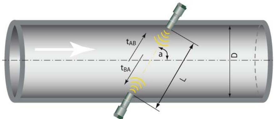
Figure 5: FLOWSIC600 measuring principle
