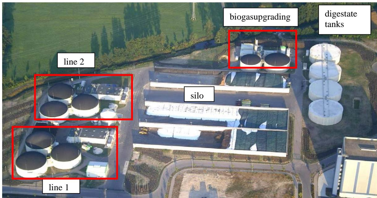
Figure 1: Aerial view of E.ON's biomethane plant Schwandorf
